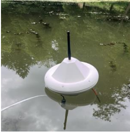
Fig. 2 — Prototype of an "autonomous" buoy built by project participants, fitted with sensors and capable of wireless communication via the LoRa protocol.
