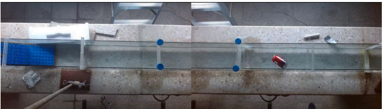
Fig. 3 — Preliminary studies of the migration of floating solid waste. The wave generator is to the right of the photo (out of frame), and the artificial beach (in blue) is on the left. During the experiment, the can moves toward the beach at an average speed that depends on its asymmetry. Left: the empty channel. Right: the can partway through its drift toward the beach.
